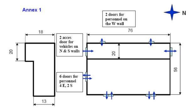
NOTE: - Sizes designate internal dimensions (inside the hangar)
