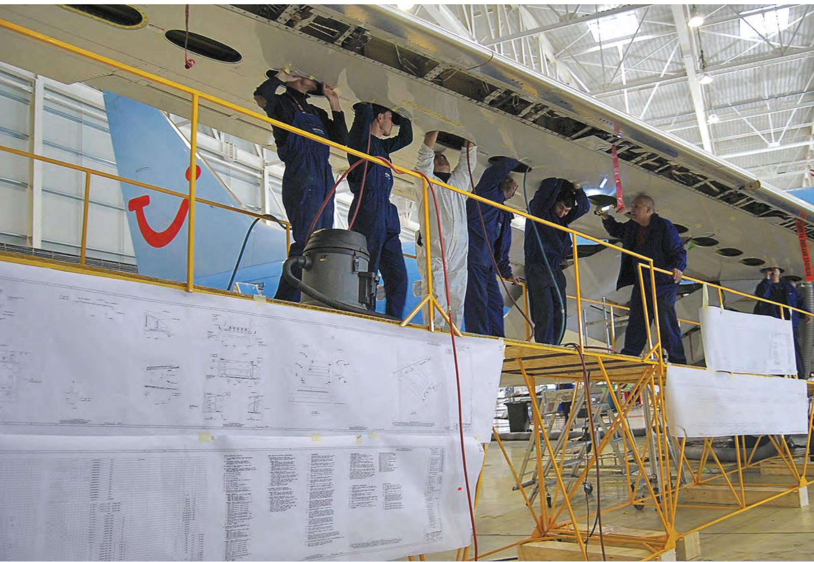
AEROSTAR provides base and heavy maintenance for commercial aircraft. The range of maintenance services was extended in 2012 to cover currently heavy checks for the AIRBUS 320 family, for Boeing 737 all series and BAe-146/ RJ aircraft and aircraft components.
